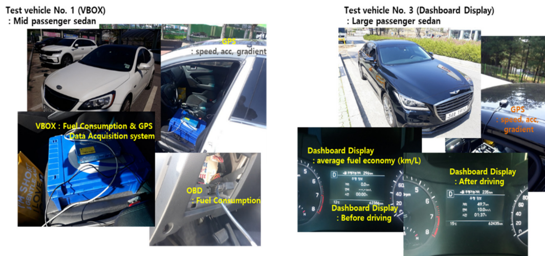
Figure 3. Test vehicle No. 1 connected to VBOX and No. 3 showing the dashboard display of fuel economy as examples.
